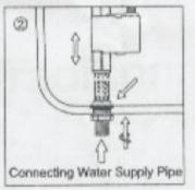
Position Valve inside tank. Push down on the Valve Shank (**Not the Top)** while tightening the lock nut. Screw the Valve Shank clockwise, and pull the Valve Body to an expected height.
