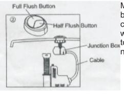
Make Cable smooth, install the button on the junction box, & then close the Tank lid, fill the tank with water & push the full & half button to check wether the flushing is normal or not.
