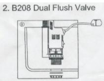
Disassemble Lock Nut, plastic washer for VALVE installation. Position the VALVE inside tank, push down on the valve body while attaching Plastic Washer & tightening Lock Nut.
